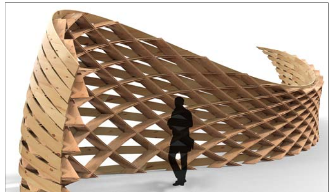
Workshop Proposal: Self-stabilizing timber frame construction through the combination of pre-fabricated elements and off-the-shelf façade planks.
